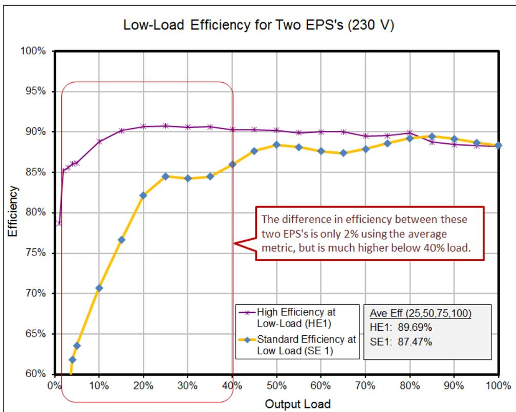
SE1 is a computer manufacturer EPS rated level V. HE1 is a Power Integrations reference design. Due to the diluting effect of the 4-point average formula, and as illustrated on this chart, a 10% load measurement is important not just for devices operating in a narrow range around 10% load, but also for all devices operating a significant amount of time below 50% load.
