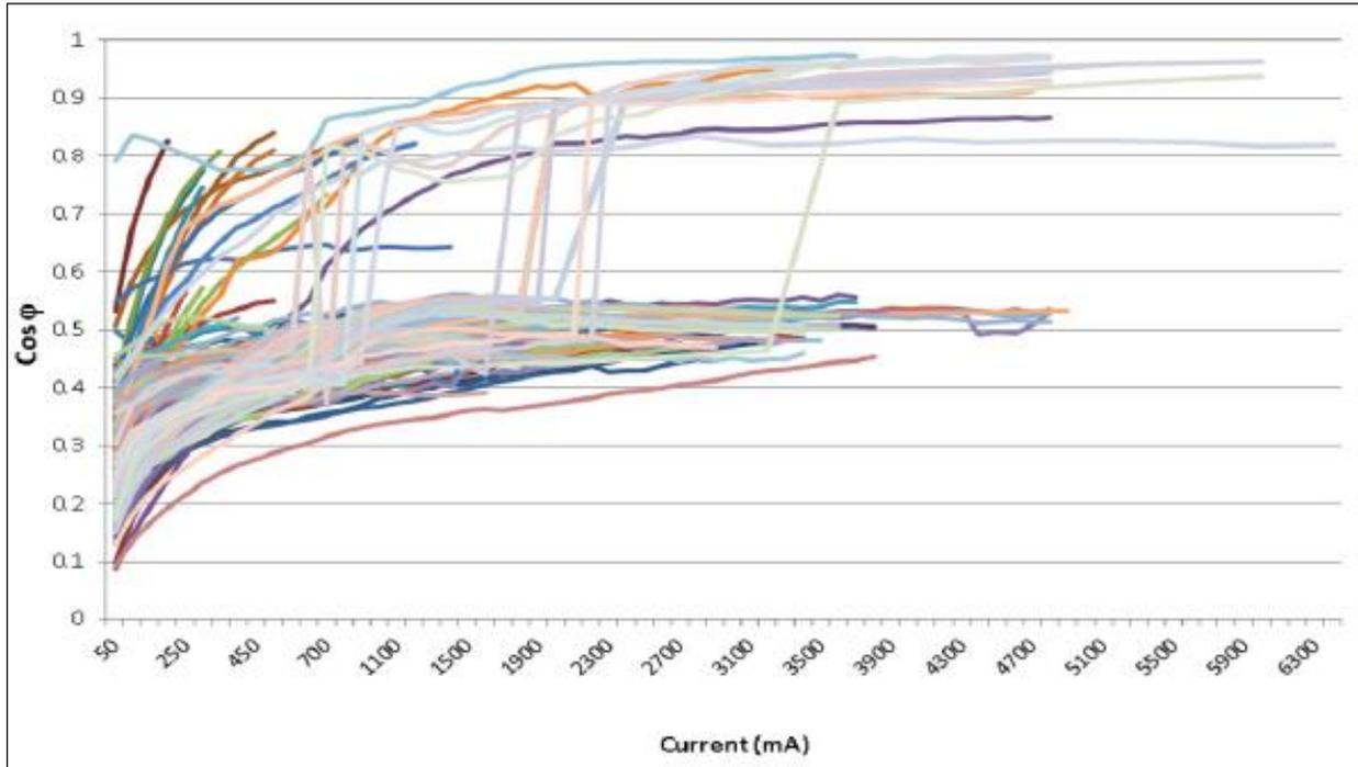
**A device with a PF of 0.4 draws 2.5 times the current compared to an ideal load with a PF of 1, which means that building wiring losses could be 6.25 times higher than the ideal case.<sup>3</sup>**
