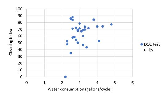
Furthermore, DOE's testing found that there are models that consume significantly less energy and water than the current standards that provide very good cleaning performance with all three soil loads. For example, Unit A, which has measured energy use and water consumption levels of 242 kWh/year and 2.8 gallons/cycle, respectively, achieved a cleaning index greater than 70 with all three soil loads.<sup>7</sup>
