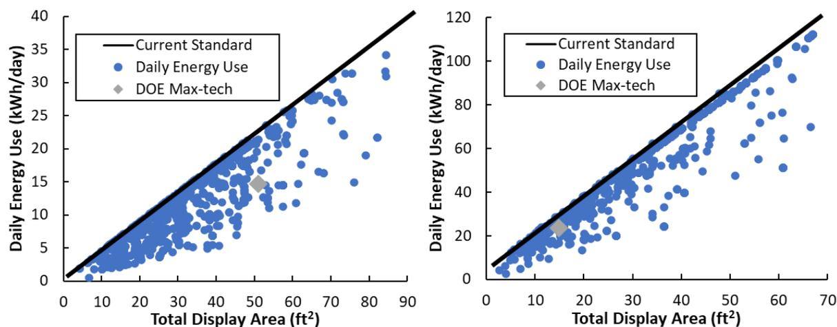
**Figure 1:** Daily energy usage (kWh/day) of SOC.RC.M (left) and VOP.SC.M (right) CREs as a function of TDA (ft<sup>2</sup>) for models in the CCD database<sup>14</sup> (blue circles). DOE’s current standard level (black line) and DOE’s max-tech level (gray diamond) are also shown.
