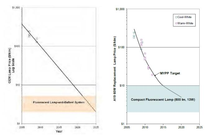
Figure 3. DOE Price Projections of LED Lamps (\$/klm) in the 2010 MYPP (left) and the 2013 MYPP (right).<sup>21</sup>
