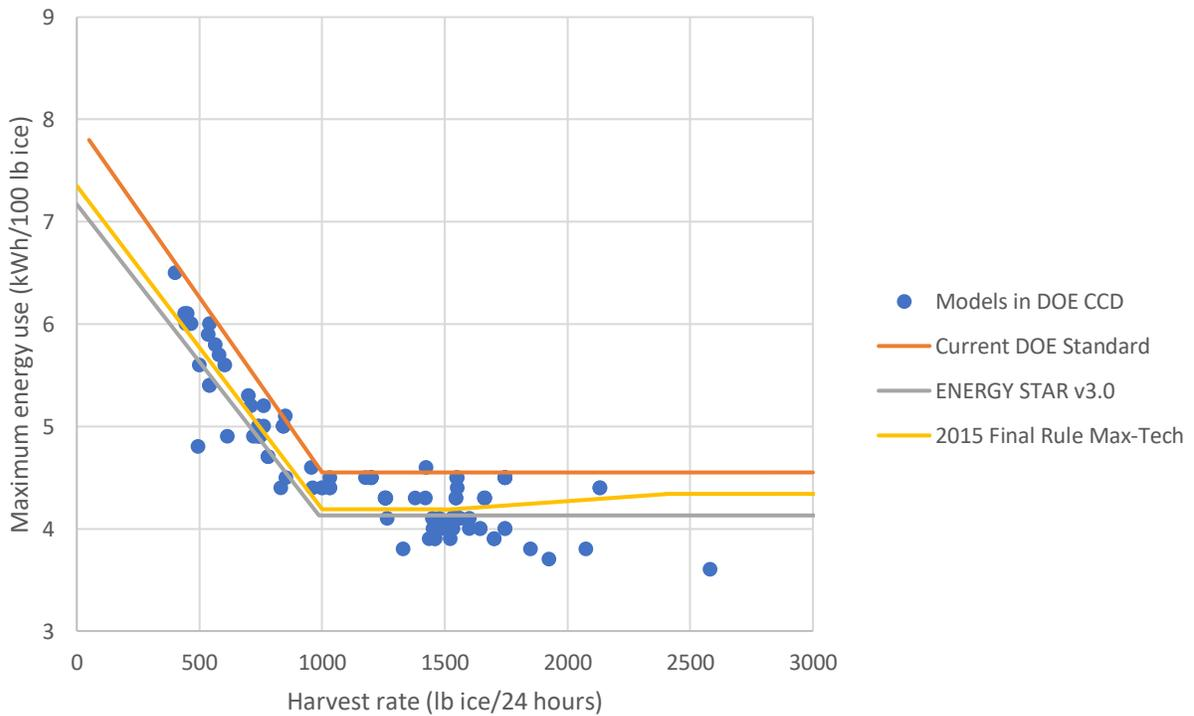
**Figure A3. Maximum energy use of batch-type air-cooled self-contained models**
