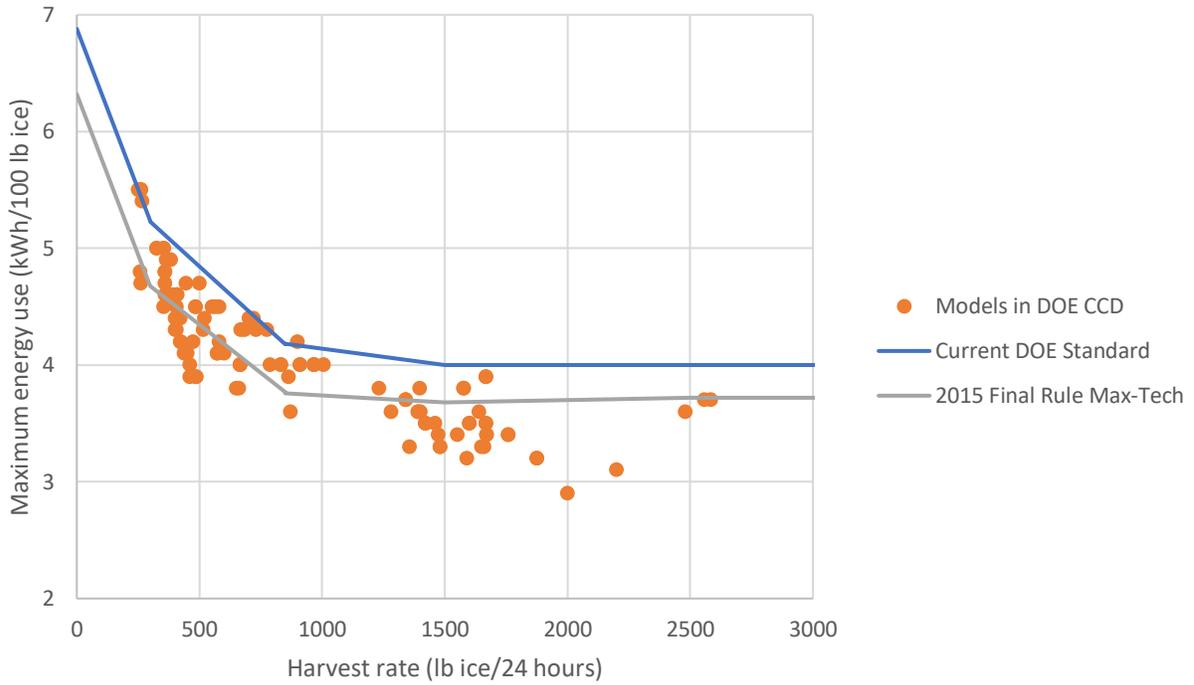
Figure A2. Maximum energy use of batch-type air-cooled remote condensing models
