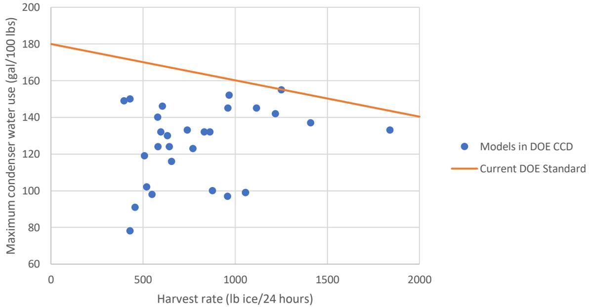
**Figure B2. Maximum condenser water use for batch-type water-cooled self-contained models**
