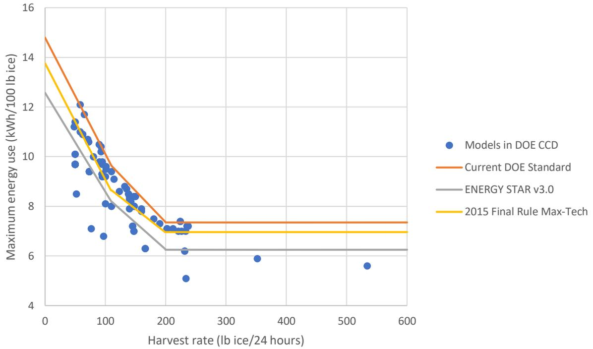
**Figure A4. Maximum energy use of continuous-type air-cooled self-contained models**
