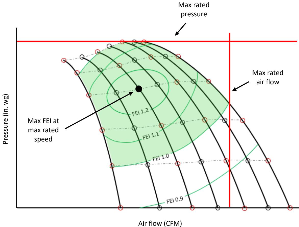
**Figure 2. Proposed approach for reporting information about a fan's compliant operating range for adjustable-pitch axial fans**
