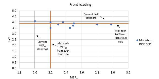
These data on available models indicate that there is significant potential to improve the efficiency of commercial clothes washers.
