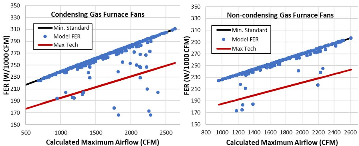
**Figure 1:** Furnace fan FER (W/1000 CFM) vs. calculated maximum airflow for condensing (left) and non-condensing (right) non-weatherized gas furnace fans. Black and red lines represent the current minimum standard and the max-tech level from the previous rulemaking analysis, respectively.
