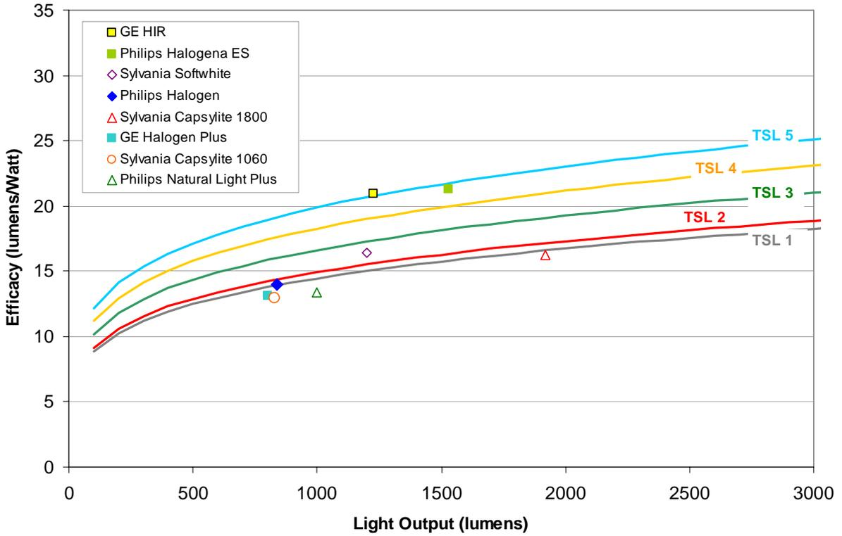
Figure 4. Modified Spectrum Lamp Test Results Compared to Modified Spectrum TSL Levels
