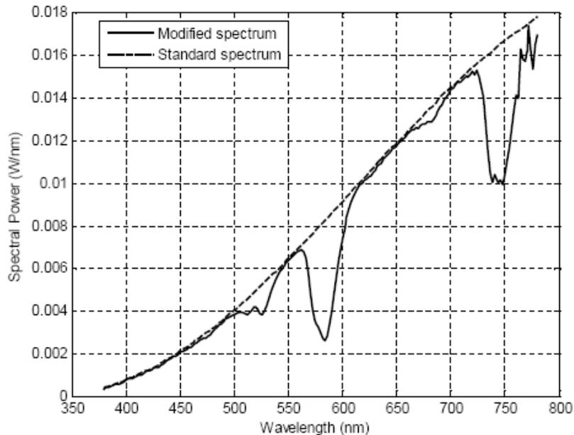
The modified spectrum effect is often created by using neodymium oxide in the glass bulb enclosure. Other types of coatings and techniques can also be used to absorb portions of the yellow, green and red wavelengths in the visible spectrum. Because, in incandescent technology, the modified spectrum effect is achieved only through filtering out portions of the spectrum, the lamp's overall efficacy is reduced.
