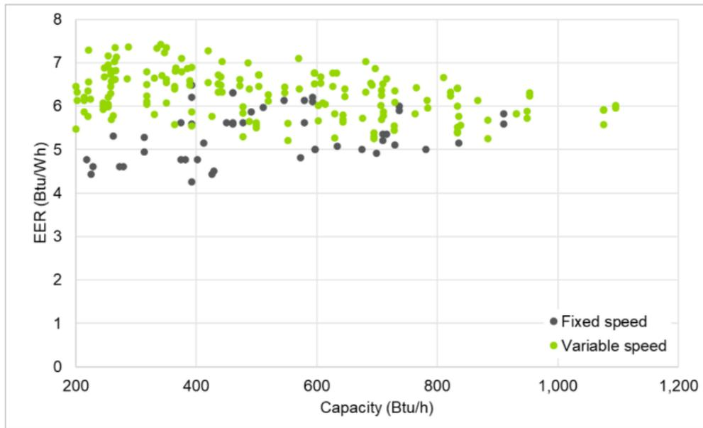
Figure 1. Efficiency Curve for R-600a Compressors (at LBP) [source: preliminary TSD Figure 5.5.1]
