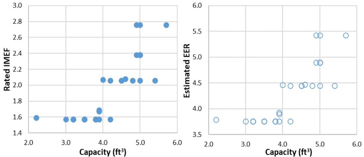
**Figure 1:** Rated IMEF (left) and estimated EER (right) versus capacity for top-loading standard washers.
